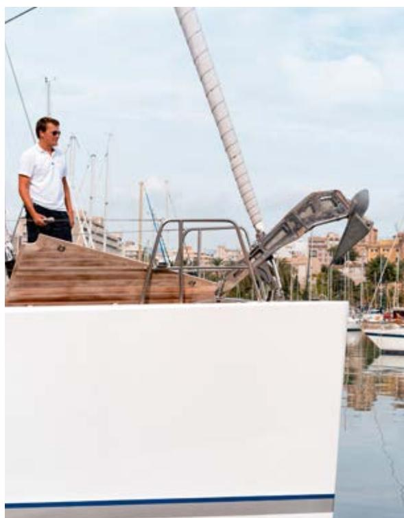
**THE ANCHOR ROLLER** and the anchor retract entirely into the anchor locker.
